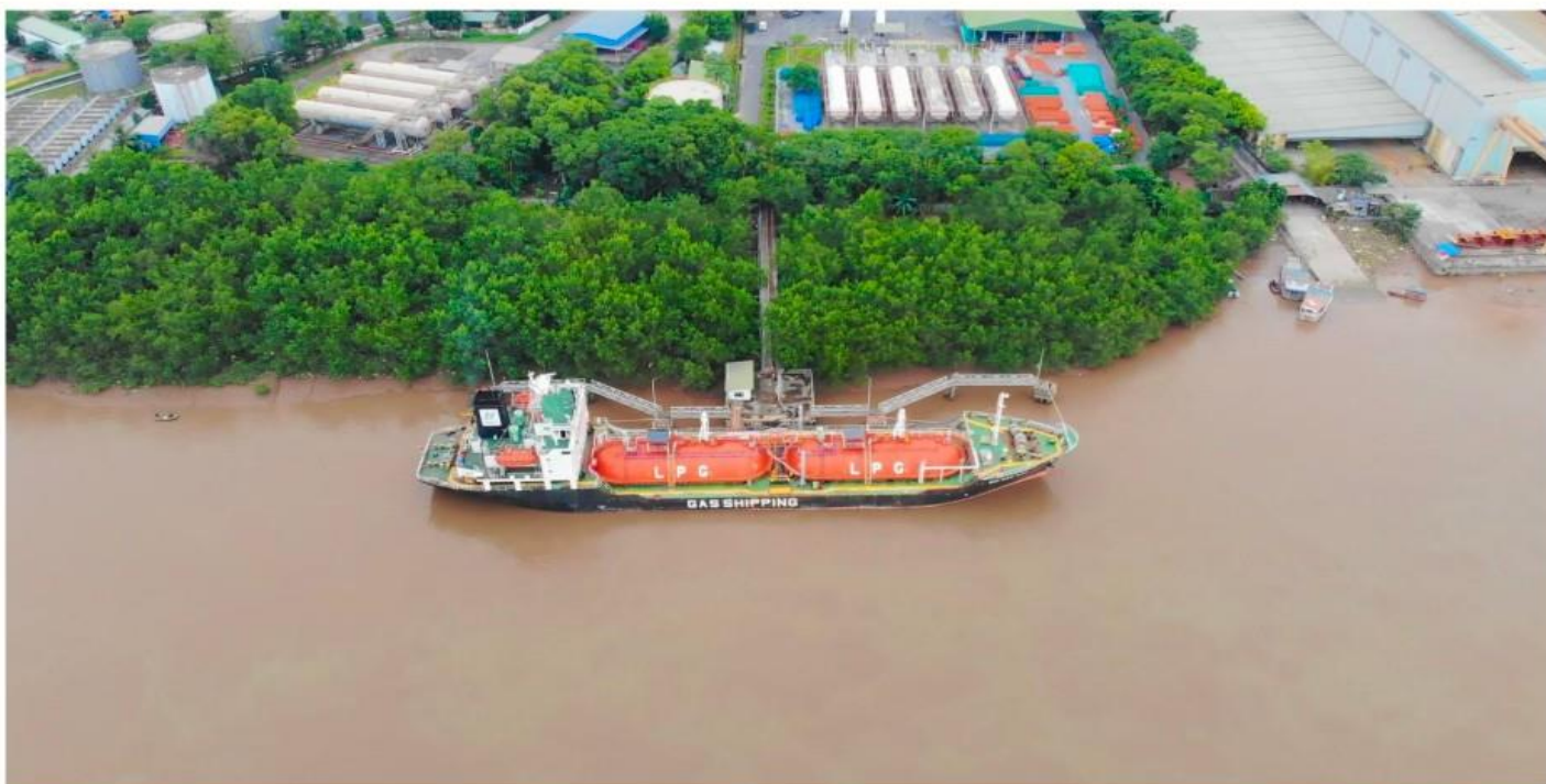
LPG JETTY (Length: 90 m, Dead Weight: 3000 DWT, Depth: -4.5 m)
